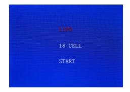
time, then display BMS24S and version, the battery type and cell count interface is displayed. Three battery pack connect to the BMS24S. Press SET/START button to run the BMS24S. After started, battery type and cell count will not be changed unless power off BMS24s. Each cell voltage and other data are displayed correctly.
